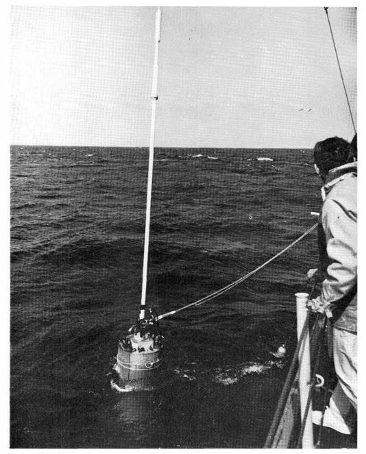
OCEAN-GOING telemetry system is this Sandia developed instrumented buoy which transmits signals from hydrophones suspended below. An array of several such buoys can be commanded from a remote control point. The antenna was designed by Phil Gelt (2624).
